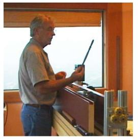
He also showed us a center rest that he made from scrap aluminum channels and some inline skate wheels which stabilized the spindle during sanding. He mentioned that h e purchased
